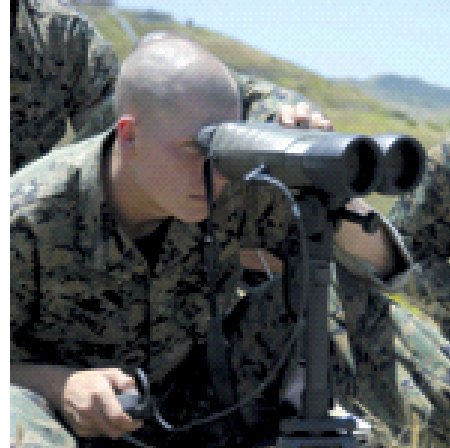
US Marines using Ashbury's VECTOR 21/CLRF and VECTOR/DAGER with remote firing switch
