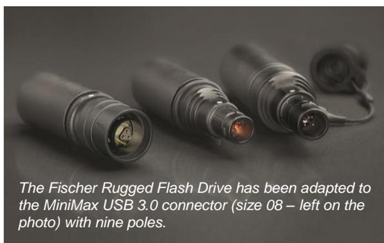
The Fischer Rugged Flash Drive has been adapted to the MiniMax USB 3.0 connector (size 08 – left on the photo) with nine poles.
